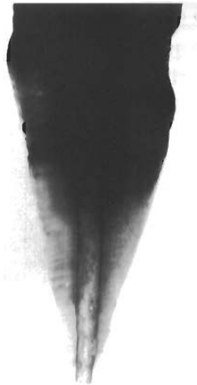
FIG 3. Cleared specimen, group C, demonstrating the extent of dye penetration after 80 days. The dye has reached the median third of the canal.
