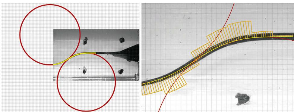
**Figure 2.** (Left) Determination of the mean radius of curvature by means of the best-fit circumference. (Right) Detail of the point-by-point construction of the mean axis of the canal (yellow). Qualitative evaluation of the curvature along the canal axis and determination of end points to determine the radius of curvature (orange).
