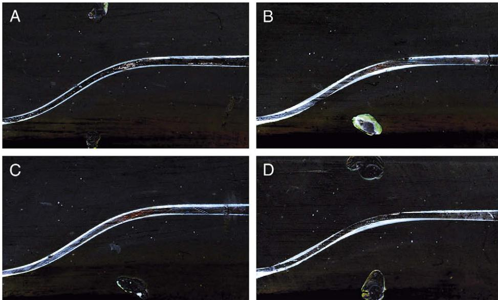
**Figure 3.** Superimposition of preinstrumentation and postinstrumentation images. (A) Group 1, PathFile/expert; (B) group 2, K-files/expert; (C) group 3, PathFile/inexpert; (D) group 4, K-files/inexpert.
